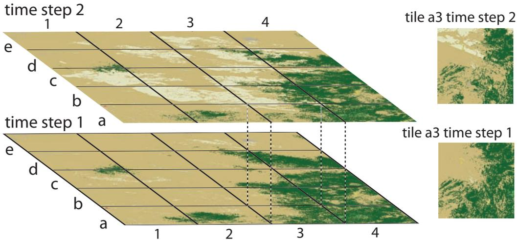
Fig. 1. The concept of pattern-based change assessment. LULC maps at two time steps are divided into spatially co-registered tiles. A dissimilarity between patterns within corresponding tiles is a measure of change. See Fig. 2 for the legend of land cover classes.
